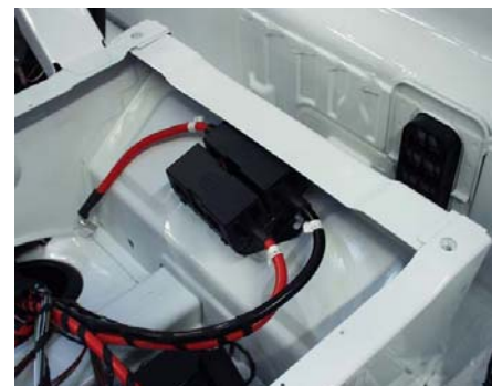
The mass cable is assembled on the rear right side of the chassis.
