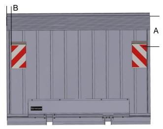
Distance A - 20 mm clearance between the open platform and the road
