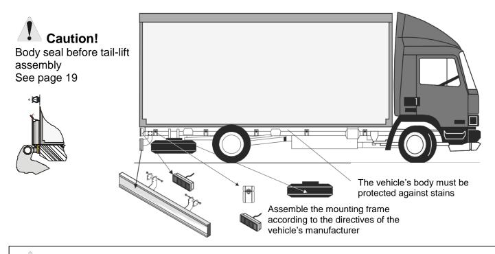
**Caution!** If the vehicle's chassis needs to be modified, the assembly directives of the vehicle's manufacturer must absolutely be respected. All and any modifications not described in these directives are subjected to written approval.
