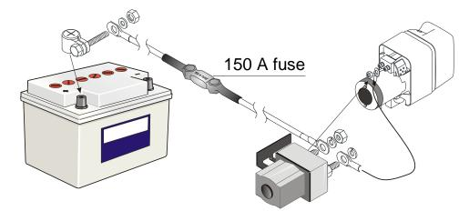
The plus and mass cables are pre-fitted on to the power unit from our factory. Lead both cables to the designated location of the vehicle. The mass cable is blue, the plus cable is red. Please ensure that there is no rubbing or pinching and that the cables do not come close to heat sources.
