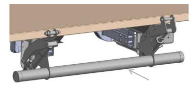
Align the left and right consoles with the adjustment fork and fasten them on to the subframe
