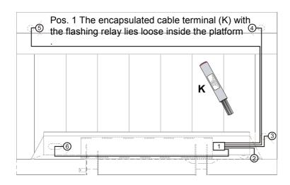
Take off the right aluminum profile. Cut the cable leading to the flashlights and the mercury switch. Take off the old cable set.
