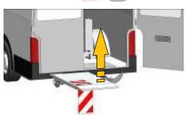
18. Lift the platform of the liftgate up till stop with the operators panel (lifting), or if you are on the platform with the foot controls or the option handheld remote (lifting).
