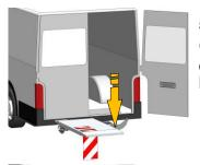
5. Lower the liftgates platform with the operating panel (lowering), or if you are on the platform - the foot control or the option handheld remote (lowering), so it gets possible to open the left door.
