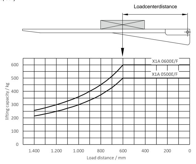
The maximum loading capacity specified in the loading diagram must not be exceeded. The platform may not be used as a bridge plate.
