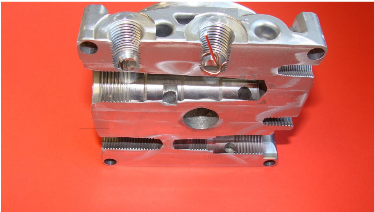
Photo 4: Valve housing sectional view
